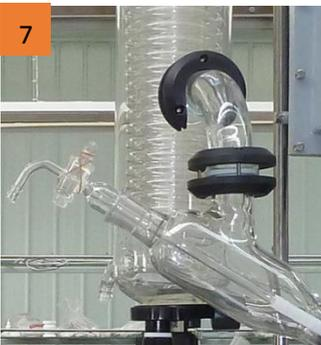
7. Bumping tube (optional) -- Preventing unexpected solution bumping into receiving flask.
