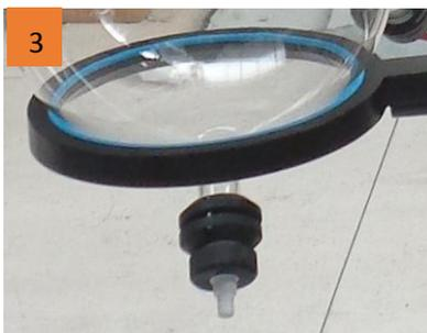
3. PTFE vacuum discharging valve -- Cork is anti-corrosion, no vacuum degree, no pollution to solvent received.
