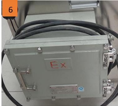
5.6. Ex-proof modification (optional) -- Offer EX proof upgrade on motor, control boxes of rotation and heating, wiring, and safety measures per user needs. Ex level reaches ExdIIBT4.
